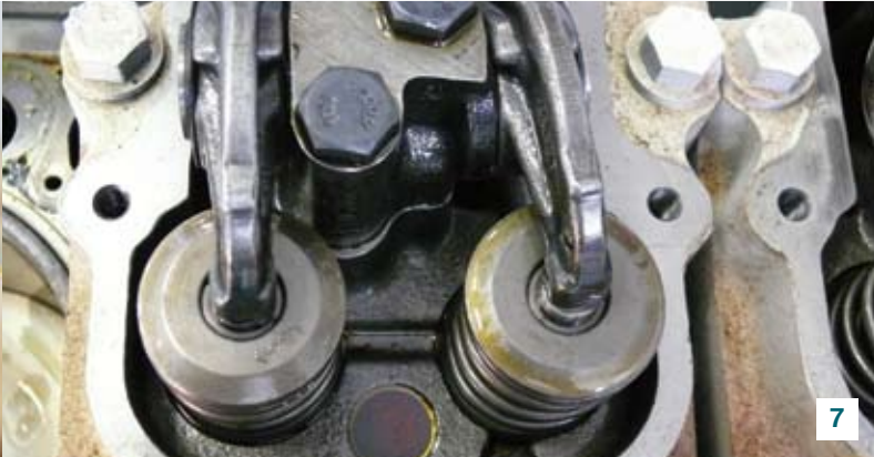
1. MAN E 2842 LE 302 V12 Piston with ring grooves; 2. MAN E 2842 LE 302 V12 Bearing shells; 3. MWM TCG 2016 V12 Piston with ring grooves; 4. MWM TCG 2016 V12 Valve train; 5. GE Jenbacher J 312 V12 Piston with ring grooves; 6. GE Jenbacher J 312 V12 Sparking plugs; 7. MTU Onsite Energy AB 3066 L4 V6 Valve train; 8. MTU Onsite Energy AB 3066 L4 V6 Inlet and exhaust valve.
